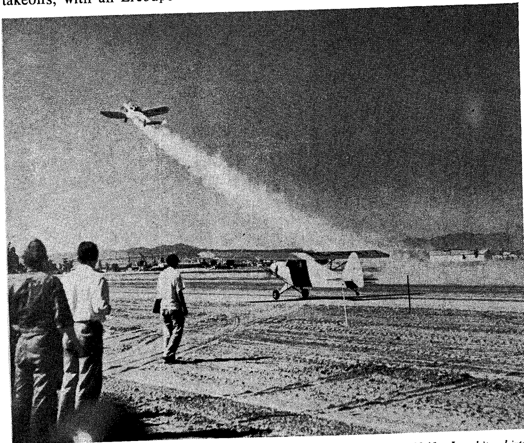
Capt. H. A. Boushey piloting 'Ercoupe' with jet-assisted take-off, August 1941. In white shirts are F. J. Malina (right) and Homer Joe Stewart. (Courtesy Caltech Engineering & Science Magazine.)
